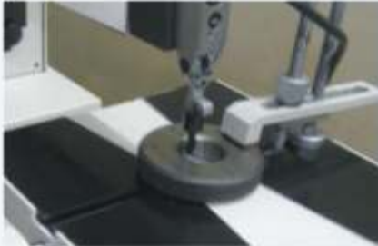
Measurement of Effective Diameter of Thread Ring Gauge
