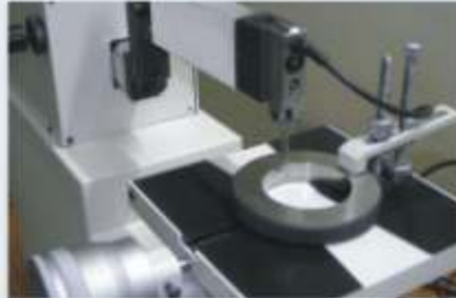
Measurement of Diameter of Plain Ring Gauge
