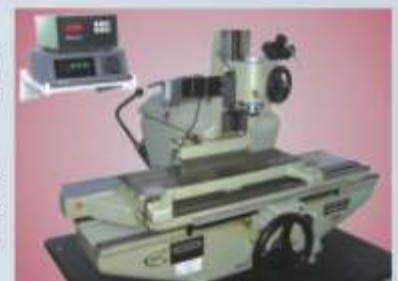
Retrofitting done for old SIP make optical universal length measuring machine MU214
